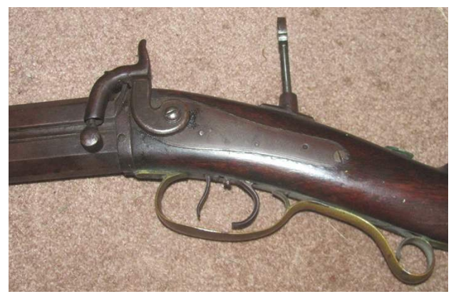
George Leonard over and under showing lollipop sight and set trigger.
