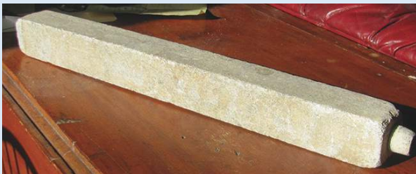
18 inch soapstone water pipe showing lead connector. PHOTO PROVIDED BY RON PATCH
