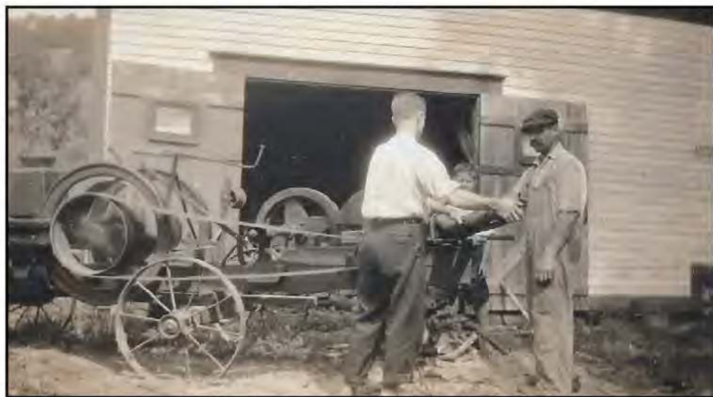
1934 Paul Richardson (left) with Mr. Richardson (right) with one-lunger machinery used to cut firewood. PHOTO PROVIDED BY CARLA WESTINE
